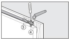
Whilst counterholding adjusting bolts
